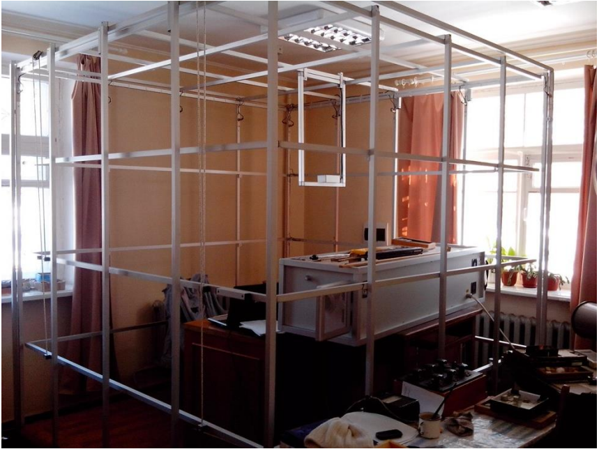
Shielded room MMLFC with high precision thermal demagnetizer MMTD and spinner magnetometer JR-6 inside the coils
