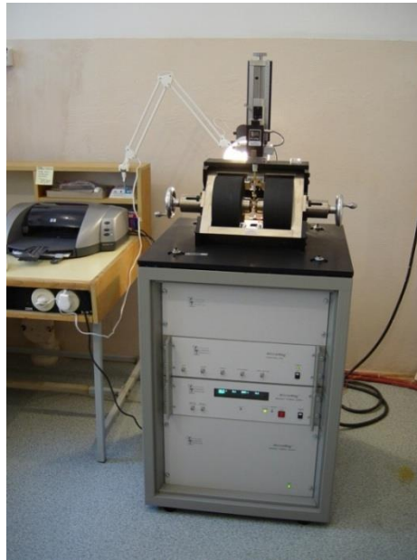
Micromag AGFM 2900-02 Alternating gradient force magnetometer
