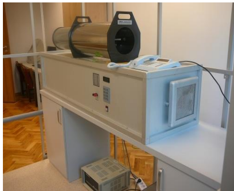
MMTD1 Nonmagnetic furnace for thermal demagnetization
