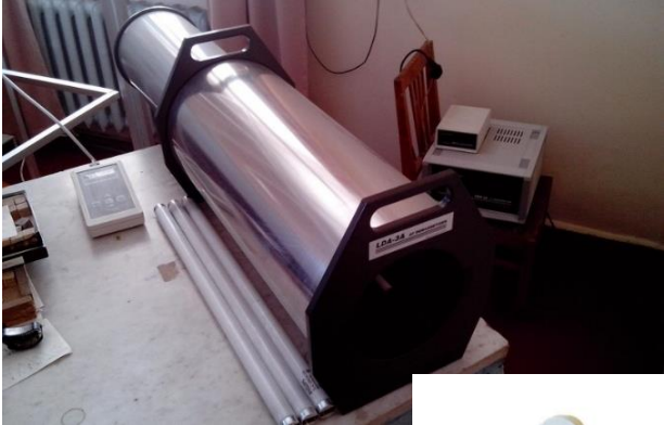
AF Demagnetizer LDA 3A with AMU-1A modul
